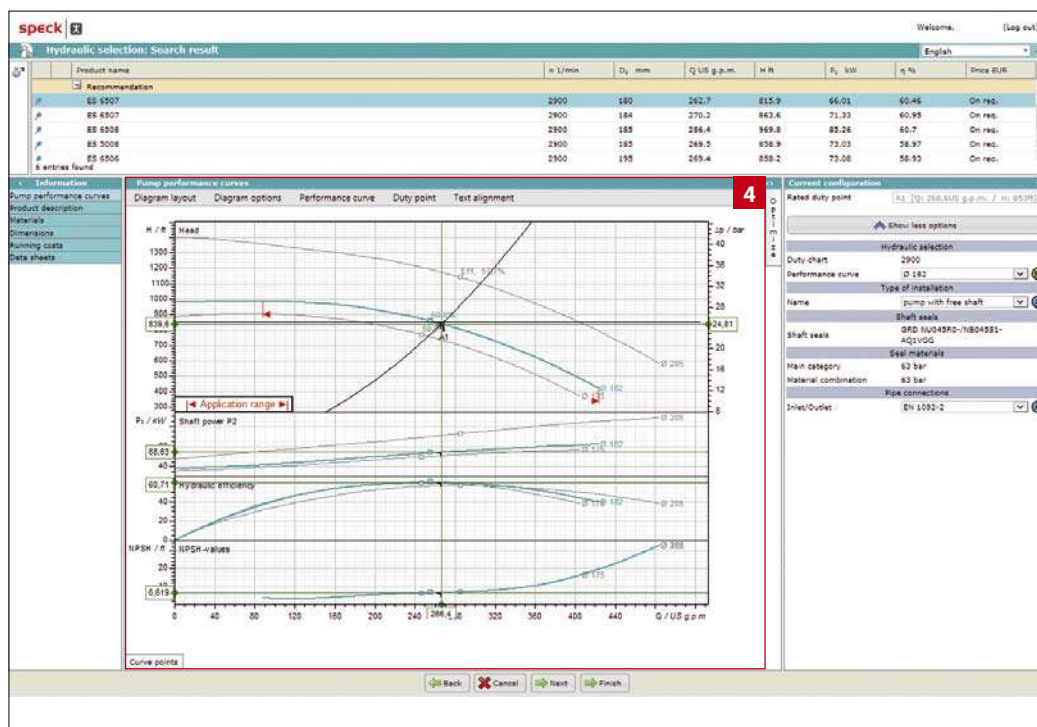
Characteristic curve depending on hydraulic selection
