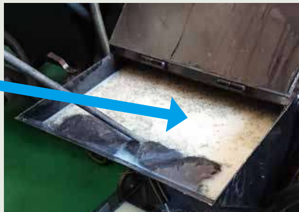
Sludge in the tank that was collected by the large flow low pressure unit.
