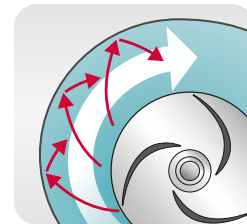
Standard impeller slams solids into the volute.
