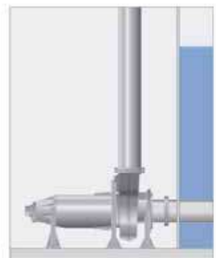
CZ - A horizontally-mounted, permanent dry well or in-line installation with flange connections for suction and discharge pipe work.
