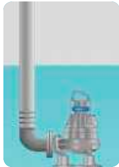
S-INSTALLATION Semi-permanent freestanding installation. Easy to transport with its pipe or hose connection.
