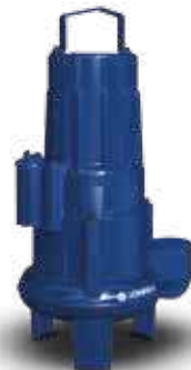
Lowara 1310 Vortex Maximum flow 16 l/s Maximum pressure 16 m Motor Rating 1.2 - 2.4 kW Outlet 50 - 80 mm Weight 46 kg
