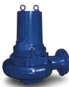
Lowara 1320 Non-clog Maximum flow 74 l/s Maximum pressure 41 m Motor Rating 3.5 - 7.5 kW Outlet 80 - 100 mm Weight 130 - 156 kg
