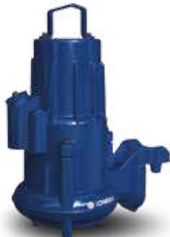
Lowara 1305 Vortex Maximum flow 10 l/s Maximum pressure 11 m Motor Rating 0.75 - 1.2 kW Outlet 50 mm Weight 30 kg
