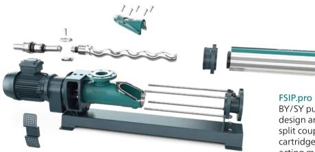
BY/SY pump with new housing design and large inspection cover, split coupling rod and 2 joints in cartridge design and MG 1 single acting mechanical seal for "Full Service in Place".
