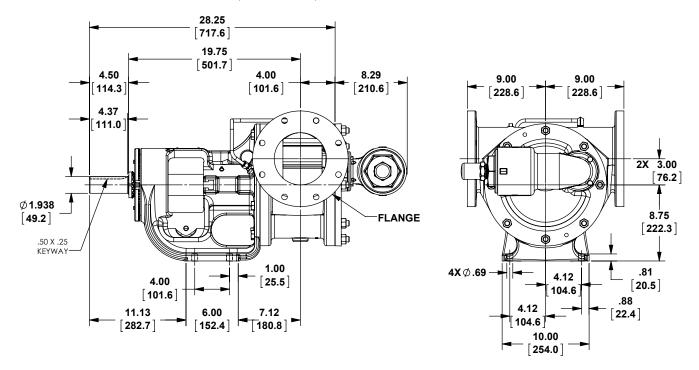
Ports are 6", suitable for use with Class 125 cast iron companion flanges or flange fittings.
