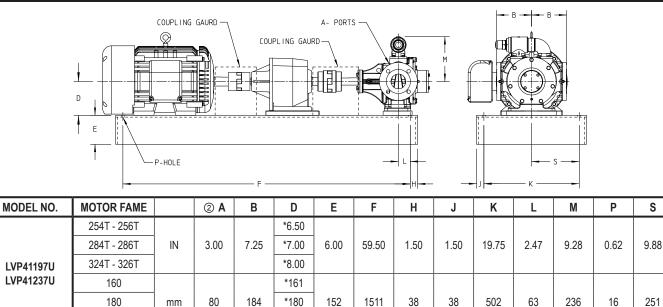
\* Dimension includes blocks under the pump and reducer. Blocks are used under the reducer, pump and motor are on the 254T - 256T frame sizes.
