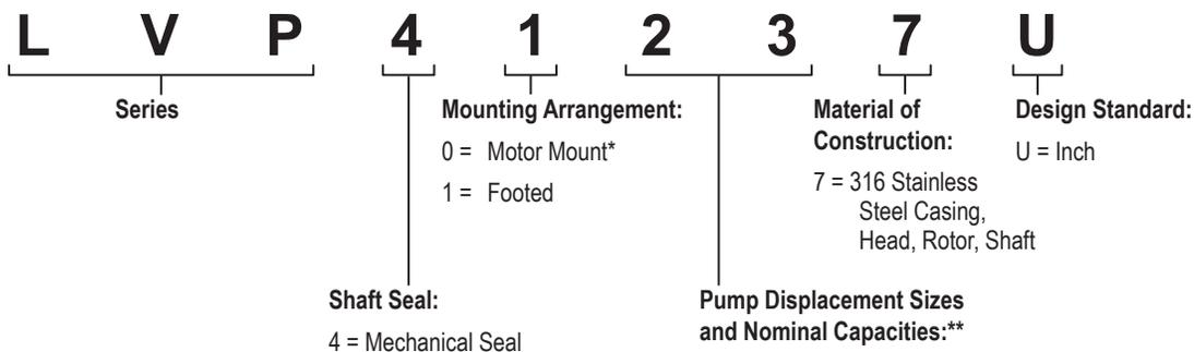
\* Motor Mount available on Displacement sizes 01 and 02 only. ANSI flanged pumps will direct mount to Nema frames 56C, 143/145TC and 182/184TC. DIN flanged pumps will direct mount to IEC B14 frames 90, 100, 112 and 132. Specify motor frame when ordering.
